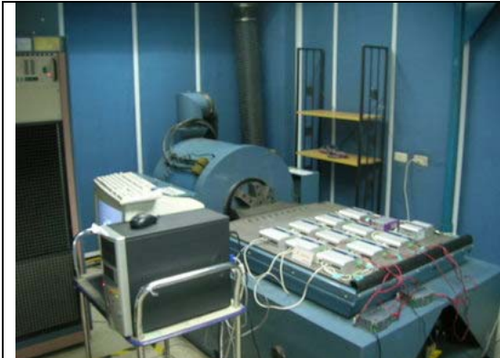
7. Operating Vibration Test --X axis
