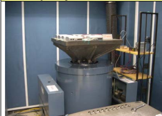
11. Operating Vibration Test --Z axis
