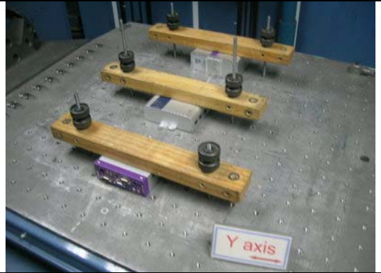
16. Non-Operating Vibration Test --Y axis
