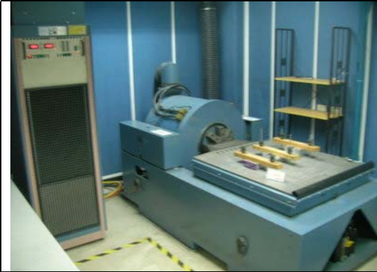
15. Non-Operating Vibration Test --Y axis
