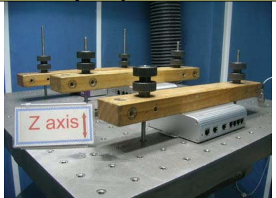
18. Non-Operating Vibration Test --Z axis
