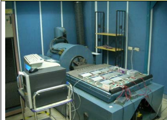
9. Operating Vibration Test --Y axis
