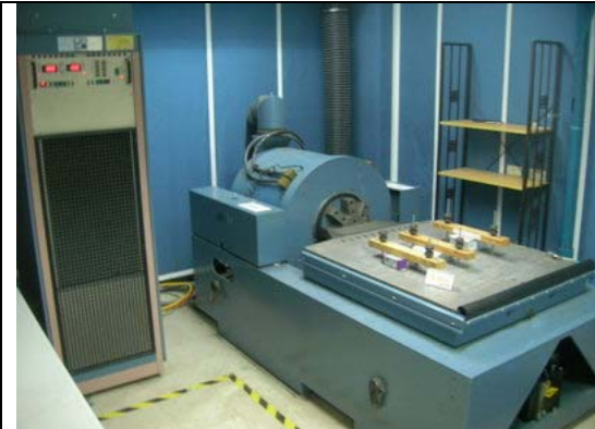
13. Non-Operating Vibration Test --X axis
