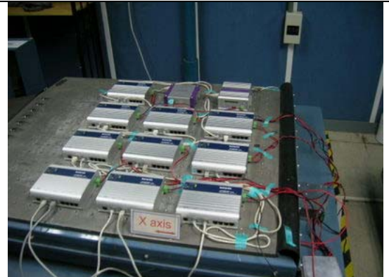
8. Operating Vibration Test --X axis
