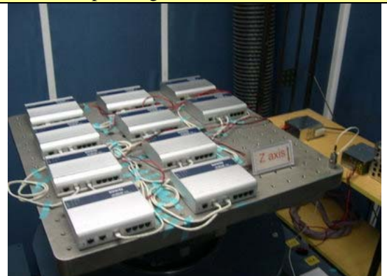
12. Operating Vibration Test --Z axis
