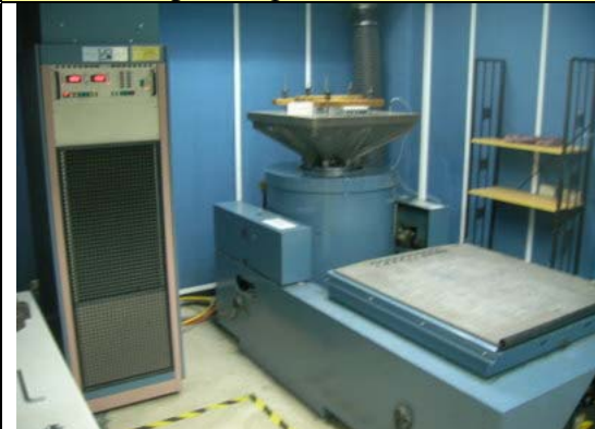
17. Non-Operating Vibration Test --Z axis
